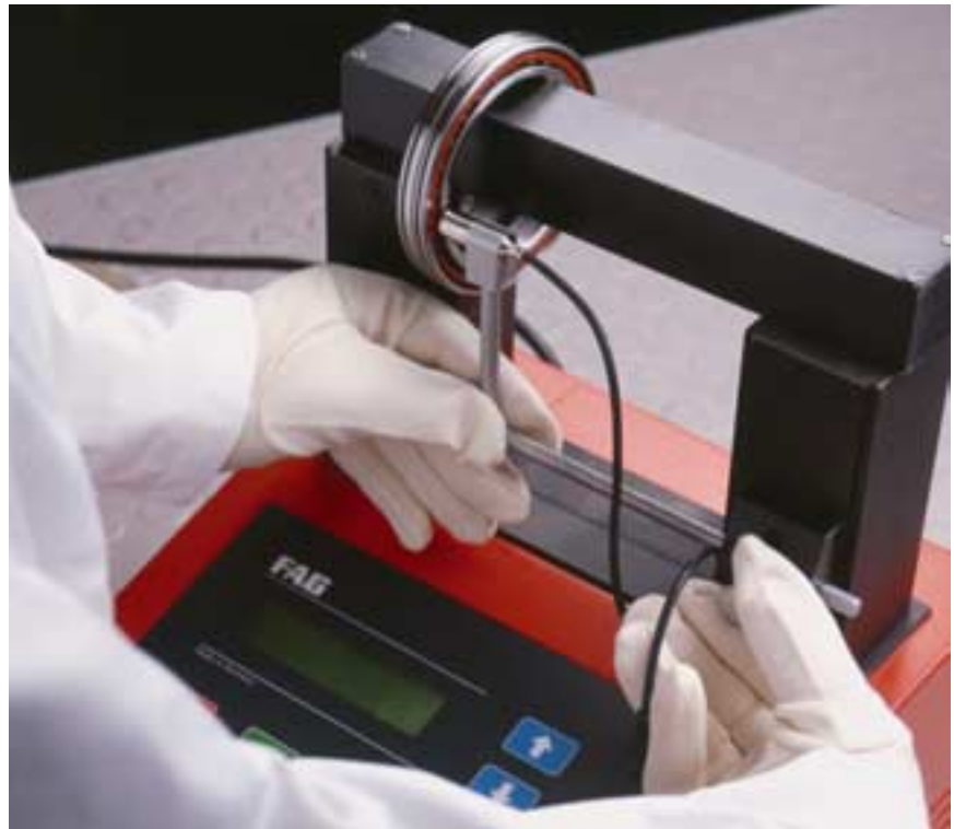
40: Mounting using an induction heating device
